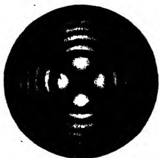
FIG. 59.—The Two Optic Axes coincident in the Centre of the Figure, two or three Minutes from the commencement. Temperature of Crystal 91^{\circ} C.
